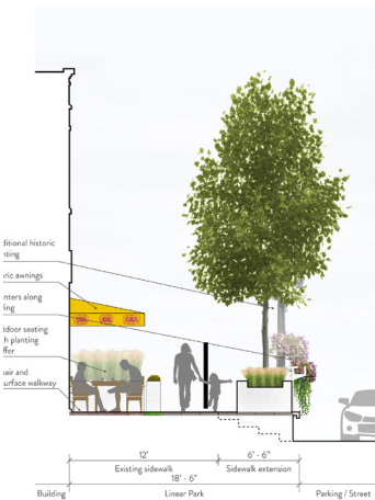
SEATING ALONG BUILDING EDGE
